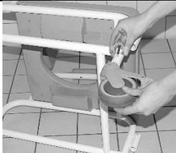
1. Lock all four wheels (by pressing down the grey plate on the wheels).
